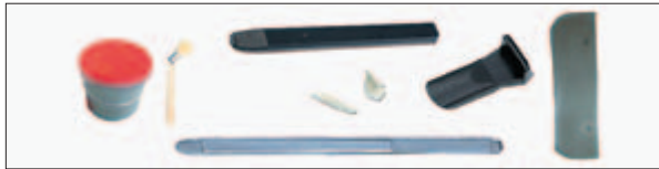
Tire paste, paste brush, bead lever and kit of plastic protectors for alloy rims
